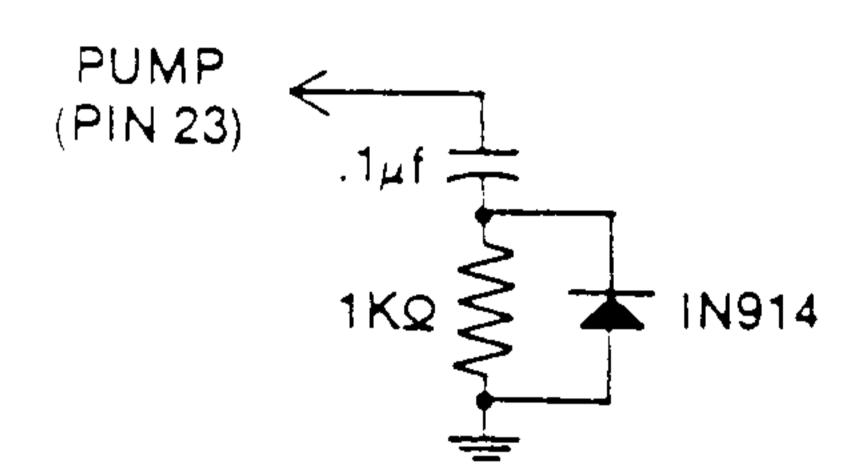
Since 5½" Drives operate at exactly one-half the data rate (250 Kb/sec) the above capacitor should be doubled to .2 or .22  $\mu$ f.
